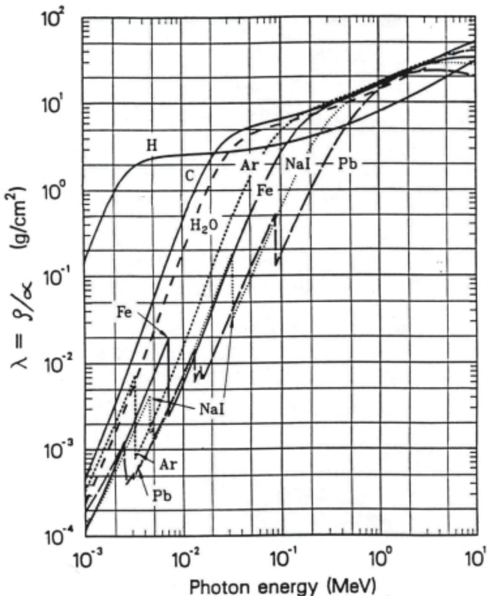
The mass absorption length  $\lambda = \rho/\alpha$  (also known as the mean free path) for various absorbers as a function of photon energy. Here  $\rho$  is the density of the absorber and  $\alpha$  is the linear absorption coefficient.
