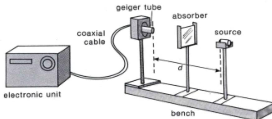
The Geiger Counter is a fragile instrument and should be handled very gently. It should remain on its stand throughout the experiment.
