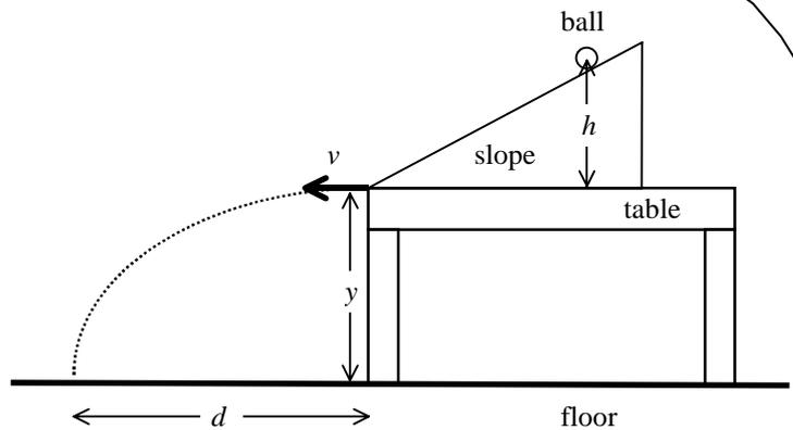
The gravitational potential energy of the ball at height  $h$  is transformed into translational kinetic energy and rotational kinetic energy. If  $v$  and  $\omega$  are the speed and angular speed, respectively, of the ball as it leaves the slope,
