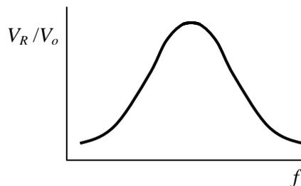
From your resonance curve, determine the resonance frequency  $f_r$ , and  $\Delta f$ , which is the full width of the curve at  $(\text{peak maximum})/\sqrt{2}$ . The  $Q$  of the circuit is then simply  $f_r/\Delta f$ .
